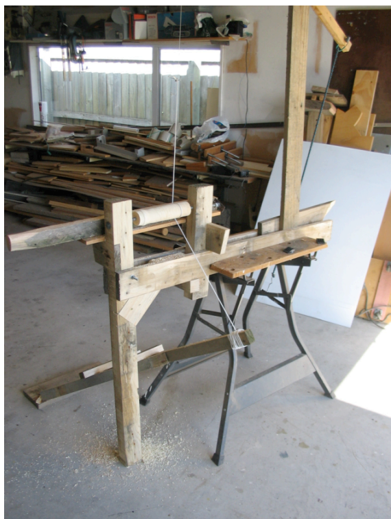
A simple hybrid pole lathe made at a class in AS XLIII
