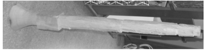
Shawm shaped with side-axe ready for final turning
